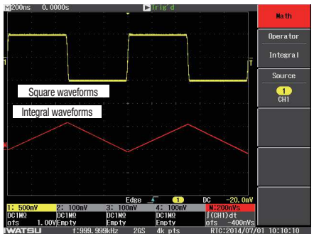
Integral calculation waveforms for square waveforms (Displays the results of integral calculus by time (∫ vdt) for the area of square waveforms.)
